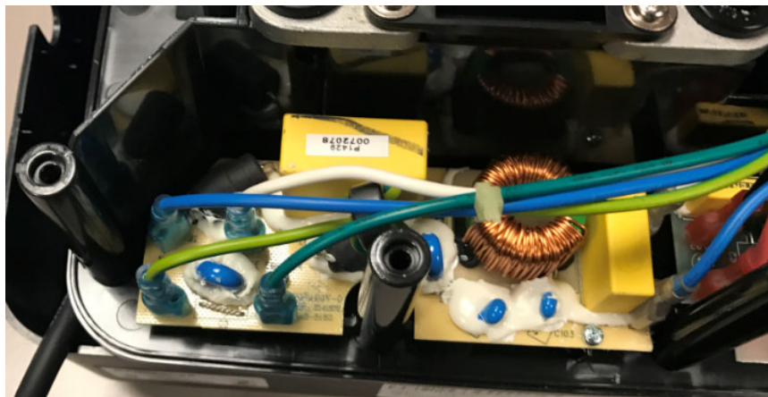
Figure 5 Interior View of RFI Board 2
