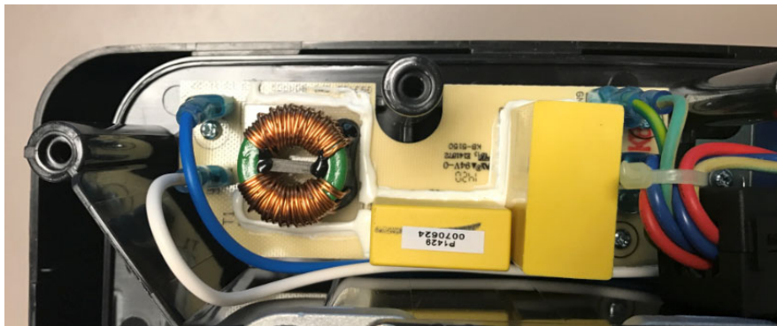
Figure 4 Interior View of RFI Board 1
