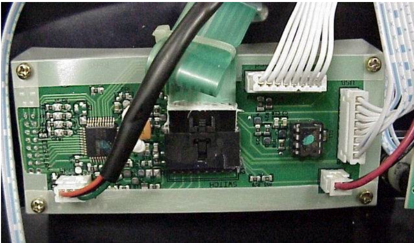
Figure 5. VFD Board (Vacuum Fluorescent Display)
