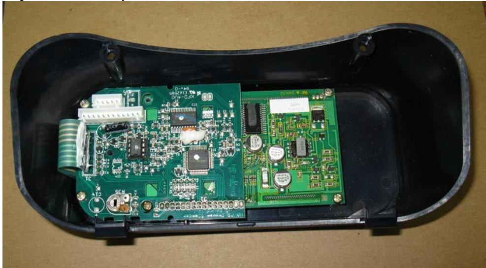
Fig. 21. Rear of Control Panel removed from unit.
