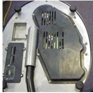
Figure 10. Cover over blender drive system.
