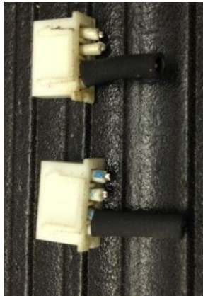
Figure 16 Heat Shrink Wrap Sealed
