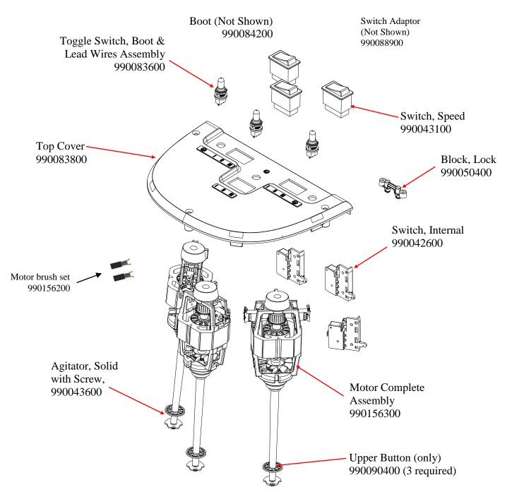
\*Switch Upgrade Kit for series A-D – 990092900 Includes: (1) Top Cover, (3) Toggle Switch, (3) Boot, (3) Grounding Wire, and (3) Switch Adaptor
