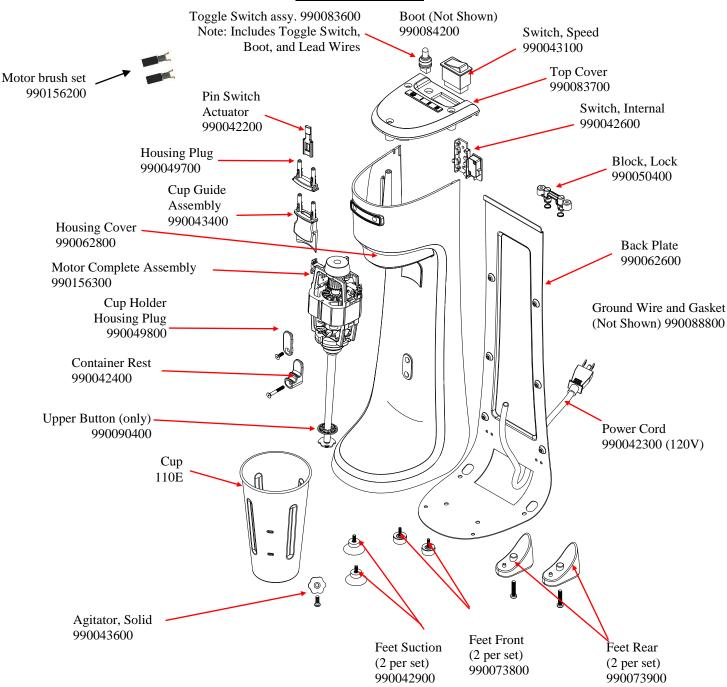
Switch Upgrade Kit (series A-D) – 990092800 Includes: Top Cover, Toggle Switch, Boot,
