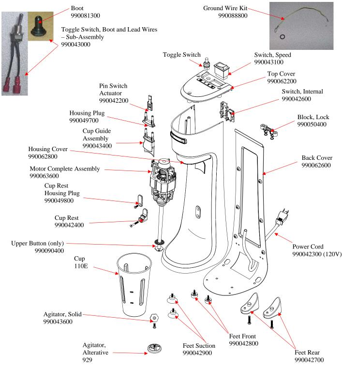
\*Switch Upgrade Kit – 990092800 Includes: Upper Lid, Toggle Switch, Boot, Grounding Wire, and Switch Adaptor
